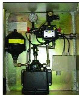
The Electric-Hydraulic Remote Control (EHR) has the same function as the EPR above, but operates a hydraulic release cylinder. Mampaey can offer either a complete hydraulic power pack or components permitting connection to the vessels hydraulic system.
